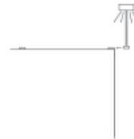
Slide light onto light base on top of frame. 1
