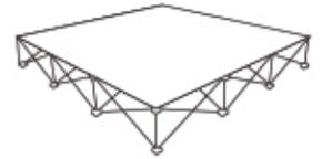
Once unit is locked, lift frame into place. \*Graphic ships pre-attached to frame 5
