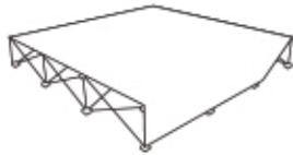
Pull end caps down to corner of frame and attach to Velcro on grey hubs. Repeat for each corner. 7
