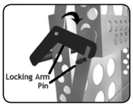
arm fit over the pin on the side of the unit.
