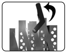
Disengage the locking arm/handle by pushing the handle toward the back of the system.
