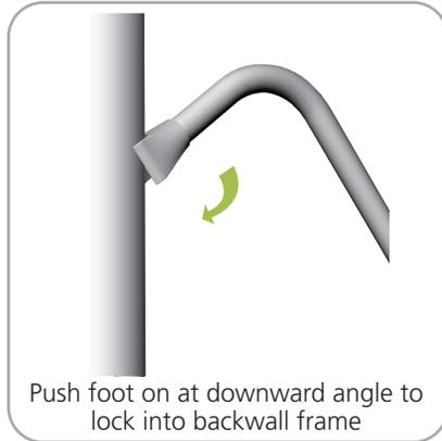
Push foot on at downward angle to lock into backwall frame
