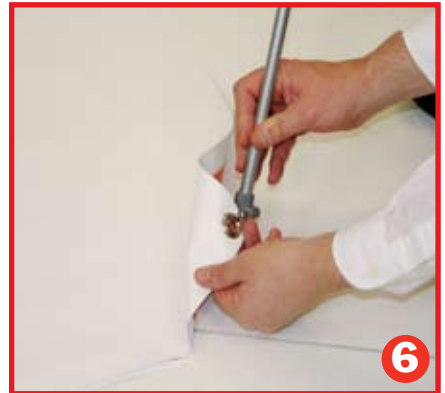
Mount the grommets, located on the bottom of the graphic, to the bottom hooks.
